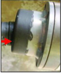
**Note:** When handling a propeller shaft out of the vehicle, it is important to support it so that the boot on the center joint is not damaged. Allowing the shaft to fold at the center joint may cause the boot to be cut by the edge of the joint.
