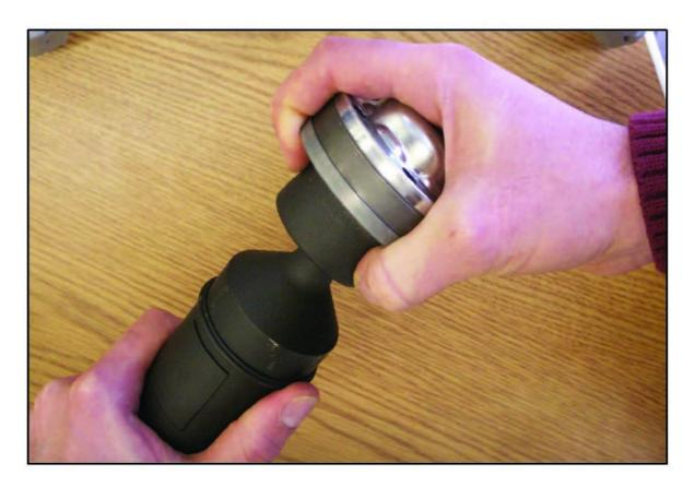
**Note:** It is normal for the front & rear joints to feel stiff when the propeller shaft is out of the vehicle. (These are not the same type of joints as the ones used on front axles.)
