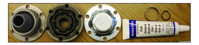
The front CV joint for original equipment propshafts on all AWD cars is now available as a spare part kit. This kit includes the boot, joint W/seals, cover, clamp, lock-ring, seals and grease.
