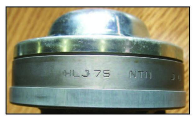
If the joint has failed, replace it according to the instructions in VIDA. Be sure to mark the rear flange of the shaft in relation to the flange on the rear axle, to prevent a vibration. Note that on some variants, different length bolts may be used at the rear for balancing purposes, and they should be installed in the same position they were removed from. The entire shaft should only be replaced if the center bearing has failed or if the tube is physically damaged.
