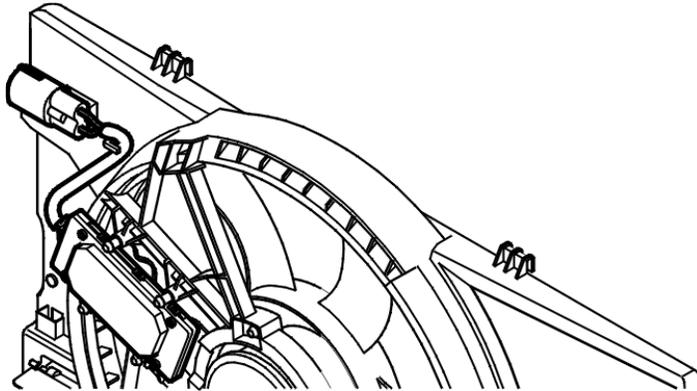
The engine cooling fan (FC) cools the coolant, engine compartment and the condenser when the air conditioning (A/C) compressor is running.
