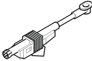
The clutch pedal sensor provides the Engine Control Module (ECM) with information about the position of the clutch pedal.
