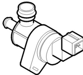
The evaporative emission system (EVAP) valve is used to open and close the connection between the EVAP canister and the intake manifold. The valve controls the flow of hydro-carbons (fuel vapor) from the EVAP canister to the engine intake manifold using the vacuum in the
