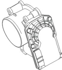
The electronic throttle unit, using the PWM control signal from the engine control module (ECM), regulates the amount of air for engine combustion. This is done using an electronically controlled shutter.
