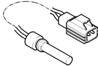
The function of the engine coolant level sensor is to alert the driver if the engine coolant level in the expansion tank is too low.
