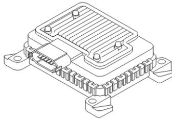
The fuel pump control module powers the fuel pump and regulates the output of the pump. The fuel pressure changes with the output of the pump.
