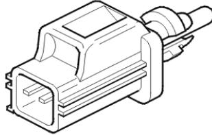
The outside temperature sensor detects the temperature in the surrounding air. The signal is used by the engine control module (ECM) as a substitute value in the event of a fault in certain components or functions and to control certain diagnostic functions.
