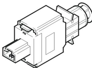
The purpose of the brake light switch is to provide the engine control module (ECM) with information indicating whether the brake pedal is depressed.
