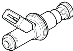
The function of the injectors is to spray fuel into the cylinders in the correct spray patterns. This happens sequentially.
