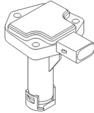
The oil level sensor provides the engine control module (ECM) with information about the quality and temperature of the engine oil and the oil level in the oil trough. Which of these functions is used by the sensor varies between different car models.
