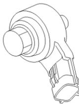
The function of the knock sensor (KS) is to monitor combustion knocking from the engine. Knocking may damage the engine and reduces the efficiency of engine combustion. If the engine control module (ECM) registers
