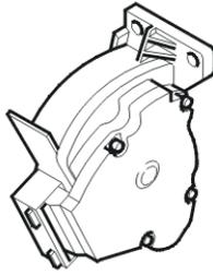
The function of the accelerator pedal (AP) position sensor is to provide the engine control module (ECM) and central electronic module (CEM) with information about the position of the accelerator pedal. This data is used by the engine control module (ECM) to deploy the shutter in the throttle unit to the correct angle.
