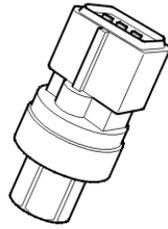
The air conditioning (A/C) pressure sensor detects the pressure in the high-pressure side of the air conditioning (A/C) system.
