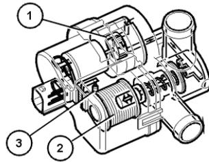
The function of the leak diagnostic unit is to pressurize the fuel tank system during leak diagnostics and to open the fuel tank system to the surrounding air during evaporative emissions control.
