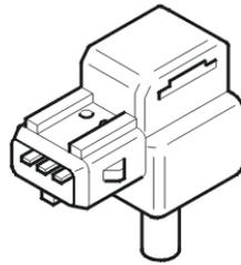
The manifold absolute pressure (MAP) sensor is on top of the radiator and is connected to the intake manifold by a hose.
