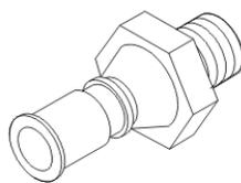
The function of the oil pressure sensor is to warn the driver about low oil pressure via the driver information module (DIM).
