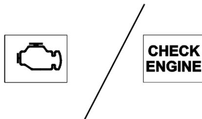
The emissions warning lamp in the Driver Information Module (DIM) has a warning symbol. This warning symbol varies
